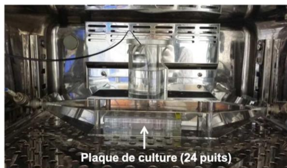
Figure 23: Culture plate (24 wells) inserted into a device housed inside a culture incubator. The device's power supply allows calibrated exposure of microglial cells seeded in culture wells to 1800MHz GSM-type signals (Credits: Michel Mallat)
