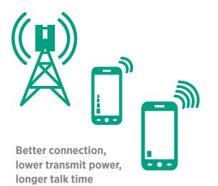
Many people do not understand how a mobile phone works. They do not understand that the phone transmits and receives radio signals and that the phone uses less power when the network connection is good, such as nearer to an antenna site.
